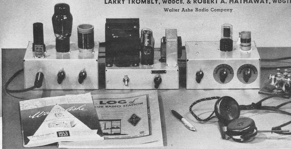
The complete Novice station: an efficient two-tube transmitter, a surprisingly effective simple receiver, and a single power supply for both. With the power supply switch in "receive" position, transmitter may be used for code practice.
